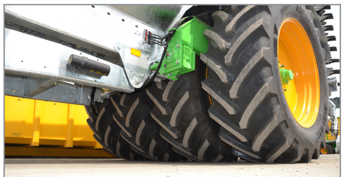
The 4 wheels of the same size in a row – 650/85R38 - \varnothing 2,070 mm – allow to uniformly distribute most of the vehicle weight to the ground.
