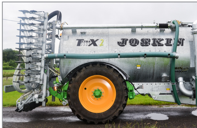
The TETRAX2 slurry spreaders are very compact and the spreading implements are hitched close to the tanker rear wall
